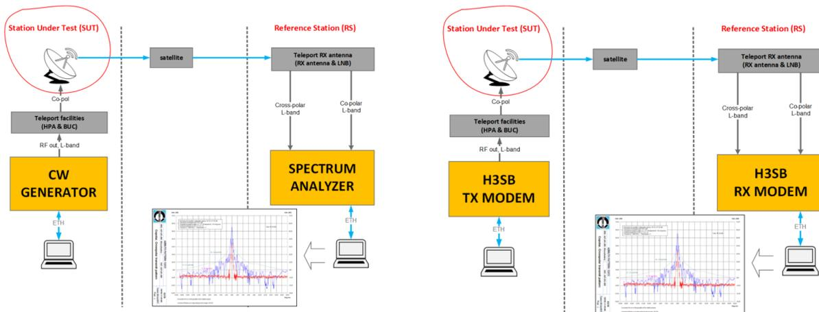
Fig. 1. The measurement process of transmitting side-lobes using a CW (left) and H3SB (right)
