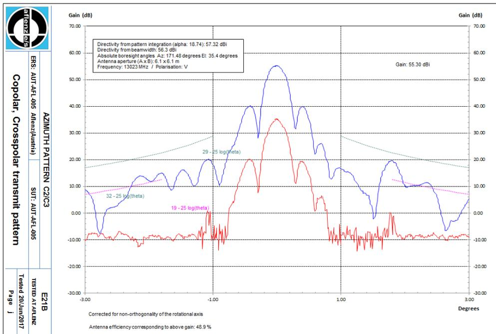
Fig. 6. The azimuth pattern, zoom in
