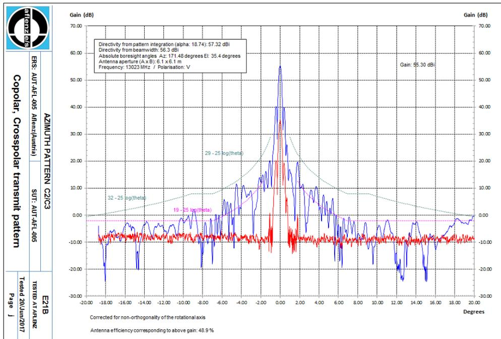
Fig. 5. The azimuth pattern
